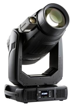
Further adding to the ground breaking RoboSpot system, the FollowSpot LT is designed for the larger venue that requires a longer throw distance, tighter beam and greater output power. The LT is the same size and weight as the standard BMFL FollowSpot, which is substantially smaller than other products of similar power. The proprietary optical design provides a 8:1 zoom ratio (1 - 8 degrees) and an output exceeding 455,000 lux at 5 metres.
